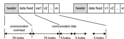
**Fig. 6.** Data transmitted in the compact format
