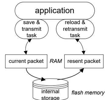
**Fig. 4.** Application tasks for data saving/retrieving on/from the device
