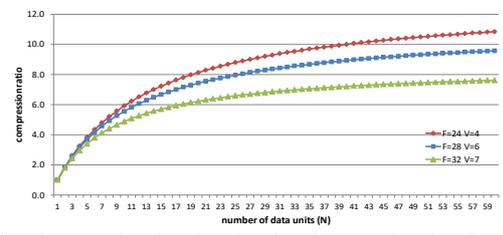
Fig. 10. Compression ratio for fix/variable data
