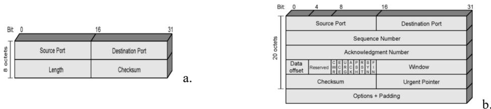
**Fig. 5.** Header format and size for a) UDP and b) TCP packets
