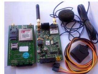
**Fig. 2.** Gipix embedded device: a. architecture; b. physical implementation.
