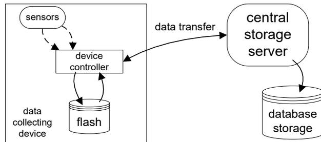
**Fig. 3.** Gipix–bird’s eye view: data storage and transmission
