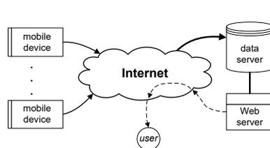
**Fig. 1.** Gipix vehicle tracking system – main architecture
