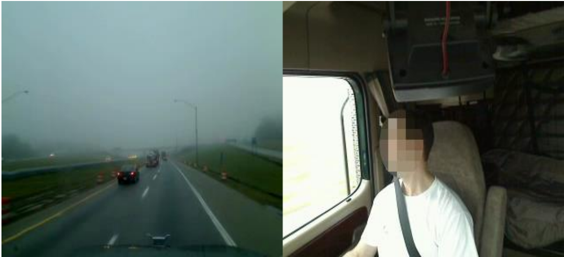
Figure 5.1: Visual Information from Internal and External Environment of the Vehicle Synchronized and Fused Together
