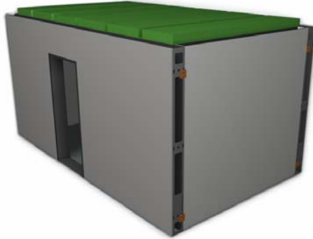
Figure 6. IFT modules are created by joining four wall panels and one ceiling form.
