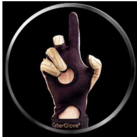
Figure 3 – CyberGlove by Immersion lifelike animations of each fingerspelled letter. Each set of captured data was saved in FBX format. This is the standard format for this motion capture system. It was then imported into Alias MotionBuilder for clean up.
