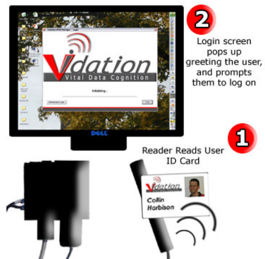
Figure 2- How the proposed RFID Login System Works
