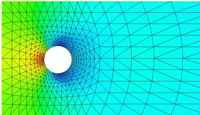
Figure 9.15 Flow around cylinder grid
