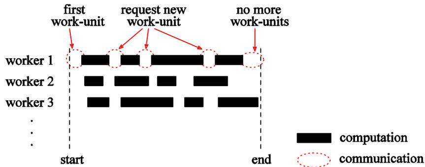
Figure 6.6 Computation times on workers: dyn. decomp-static distrib
