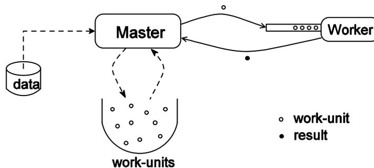
Figure 6.10 Pipelining of worker tasks
