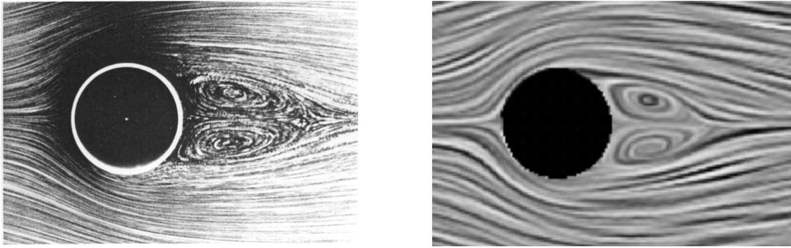
**Figure 9.16 Flow around cylinder (measurement and simulation)**
