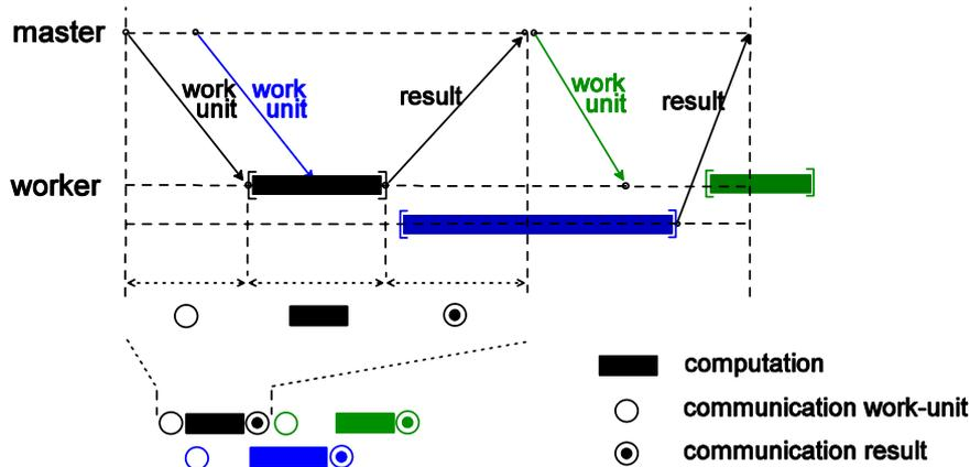
Figure 6.11 Worker timeline for unit pipeline
