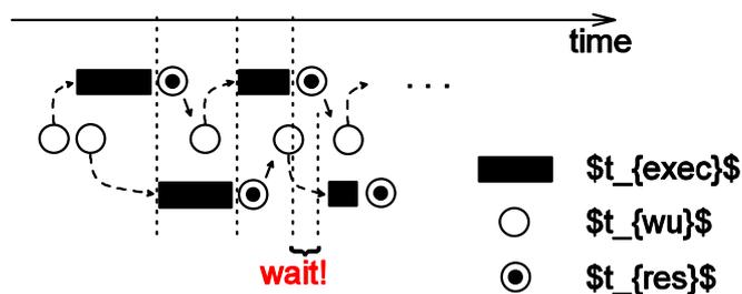
Figure 6.12 Unit pipeline - worst case
